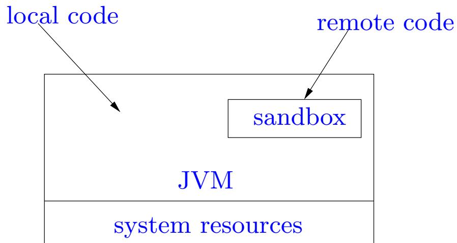
The **sandbox** principle: each application has access to a restricted set of **system resources** like local files, network, etc.
