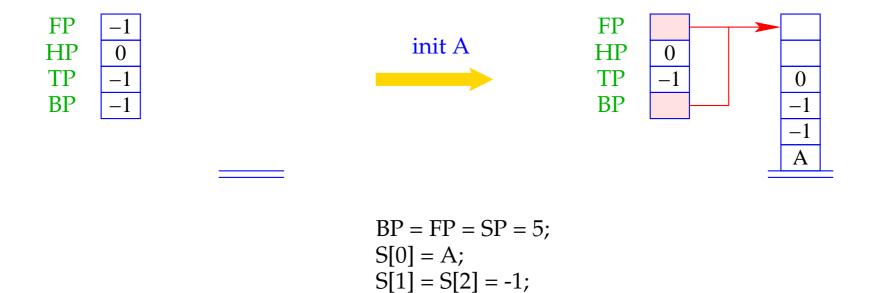
At address "A" for a failing goal we have placed the instruction no for printing no to the standard output and halt :-)
