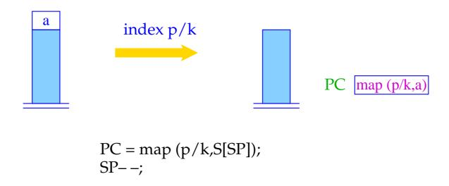
The function map() returns, for a given predicate and node content, the start address of the appropriate try chain :-)
