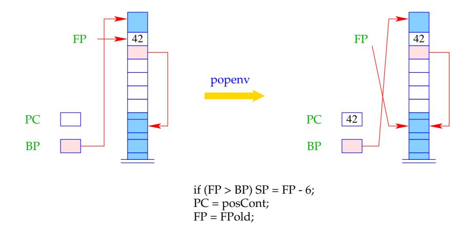
If popping the stack frame fails, new data are allocated on top of the stack. When returning to the frame, the locals still can be accessed through the FP :-))
