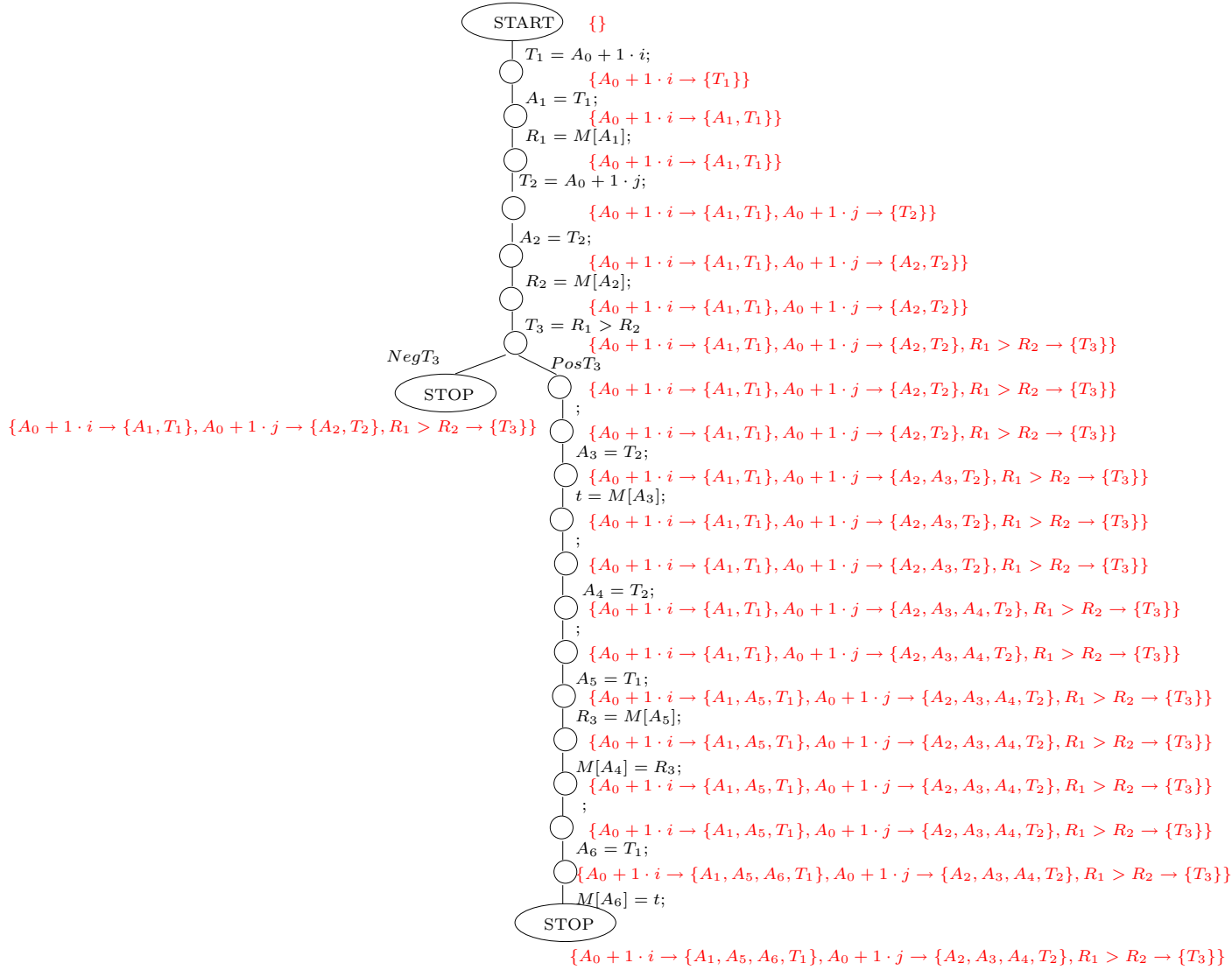
Abbildung 6: Computation of which variables contain which value.
